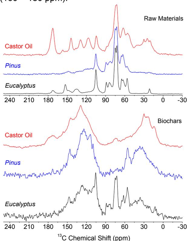
**Figure 1.** <sup>13</sup>C NMR spectra of the raw materials, castor oil cake, *Pinus* and *Eucalyptus* saw dust (top), and of the samples in the same order submitted to treatment of pyrolysis as described in the text (bottom).
