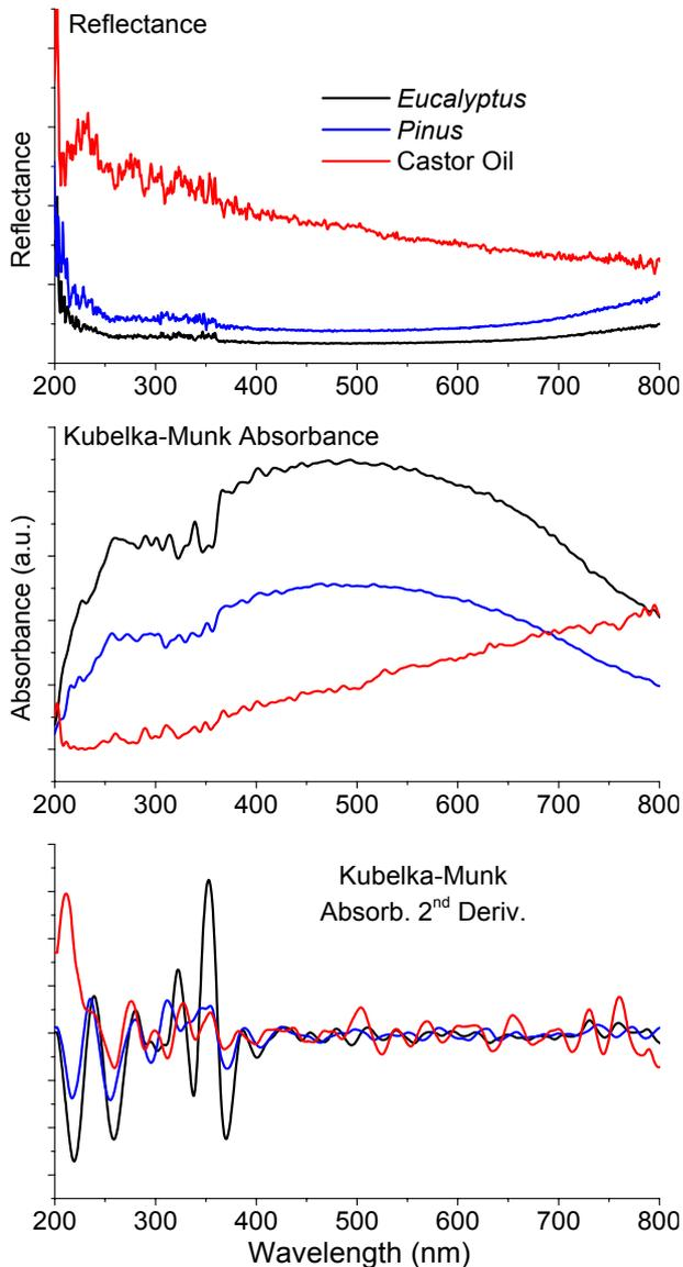
**Figure 2.** Reflectance spectra of the *Pinus* saw dust, PN4, *Eucalyptus* saw dust, E4, and castor oil cake, P4, after the pyrolysis treatment (top), Kubelka-Munk absorbance (center), and K-M second derivative mode (boton).
