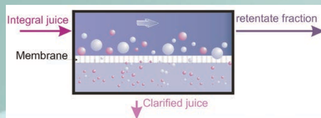
Fig. 1. Scheme of microfiltration process
