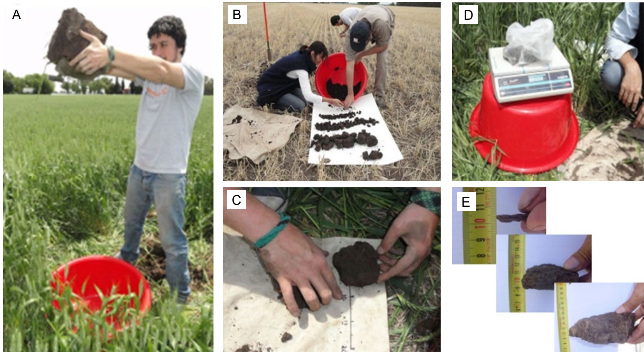
Figure 11. Illustration of the steps for the Field Visual Evaluation of Soil Structural Quality (VESS) in Argentina. A) “Burst testing”; B) Sorting soil fragments into size categories; C) Weighing each soil aggregate size fraction; D) Measuring the thickness of representative soil structural units; E) Evaluation of laminar soil structure.
