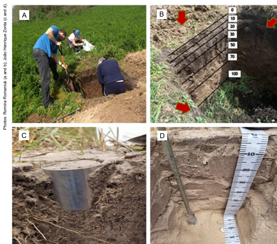
Figure 5. Illustration of methods to evaluate climate regulation SES indicators. A) Pit at 1 m soil depth; B) Depths delimited within the pit for soil sampling, the red arrows indicate that samples must be taken from three sides of the pit; C) Soil bulk density measurement by simple metallic ring at the first soil layer; D) Auger used to collect disturbed samples, and volumetric cylinders to collect undisturbed samples at the bottom soil depth.
