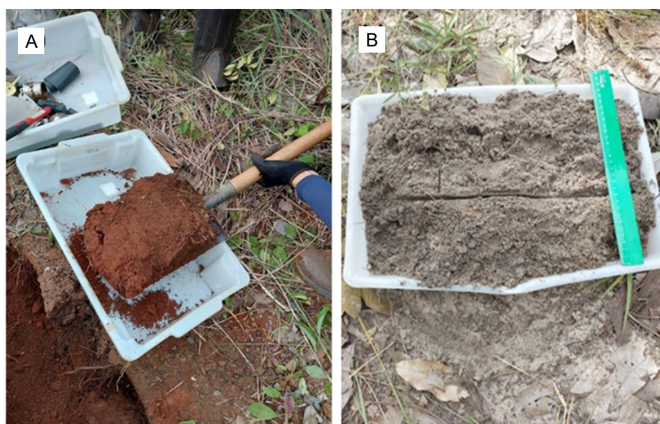
Figure 7. Illustration of RDSE methodology protocol for soil structural quality evaluation in Brazil. A) Soil block for RDSE collected with a flat shovel; B) Aggregates prepared for the evaluation of structural quality, showing the two layers where the assessment of the structural quality of the layer is conducted.
