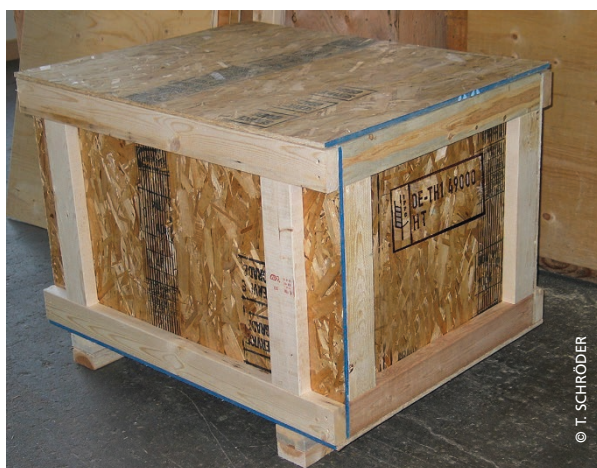
An example of wood packaging material in the United Kingdom that is subject to ISPM No. 15: it is composed of both raw wood (falling under ISPM No. 15) and processed wood (not falling under ISPM No. 15). For easy reading, the mark may be displayed on the processed wood
