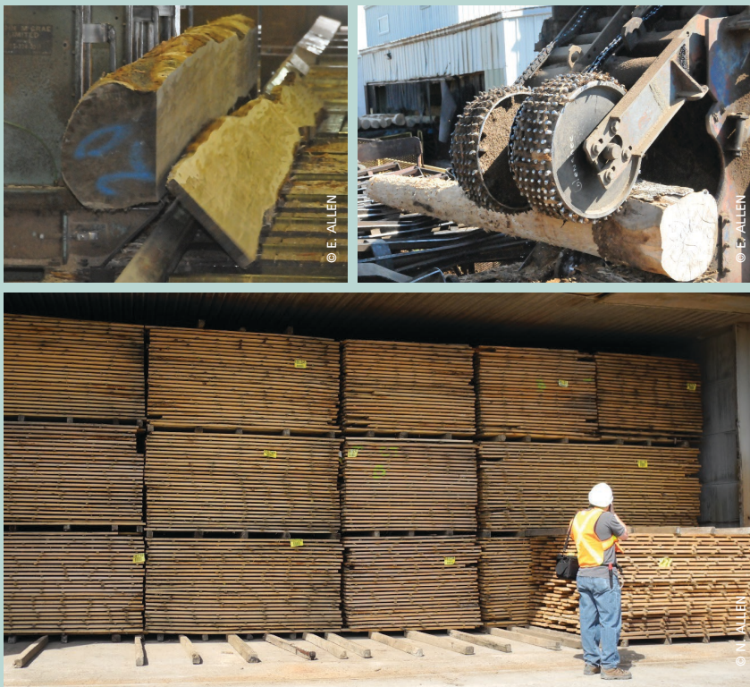
Processing ash logs at a sawmill in Ontario, Canada, in preparation for export. Top left: ash logs are debarked; top right: ash logs are sawn into boards; and boards are treated with heat in a kiln
