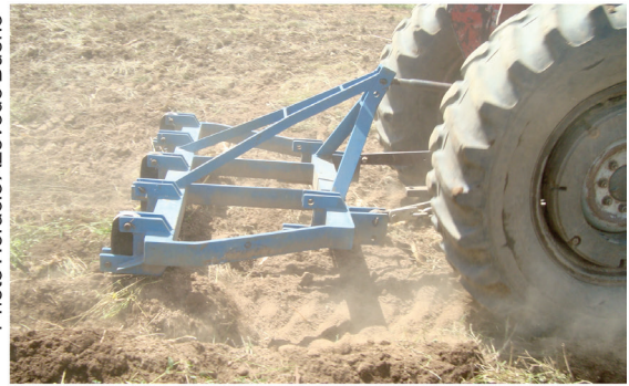
B. Cross-scarifying in soil with moisture equivalent to the point of friability.
